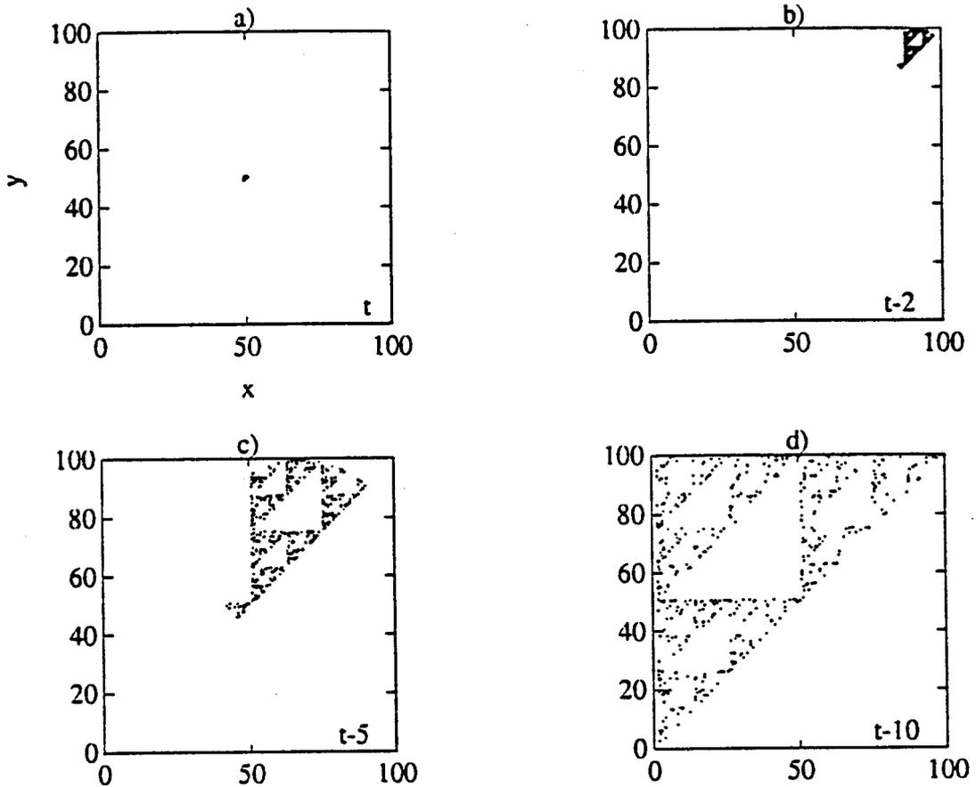
Fig. 1. In a) we consider a ball of initial conditions at time  $t$  of radius 1; b), c) and d) show how this set evolves after 2, 5 and 10 backward iterations under the action of the chaotic shift dynamical system (21). The quasi-totally disconnected (just-touching) IFS used in these simulations is:
